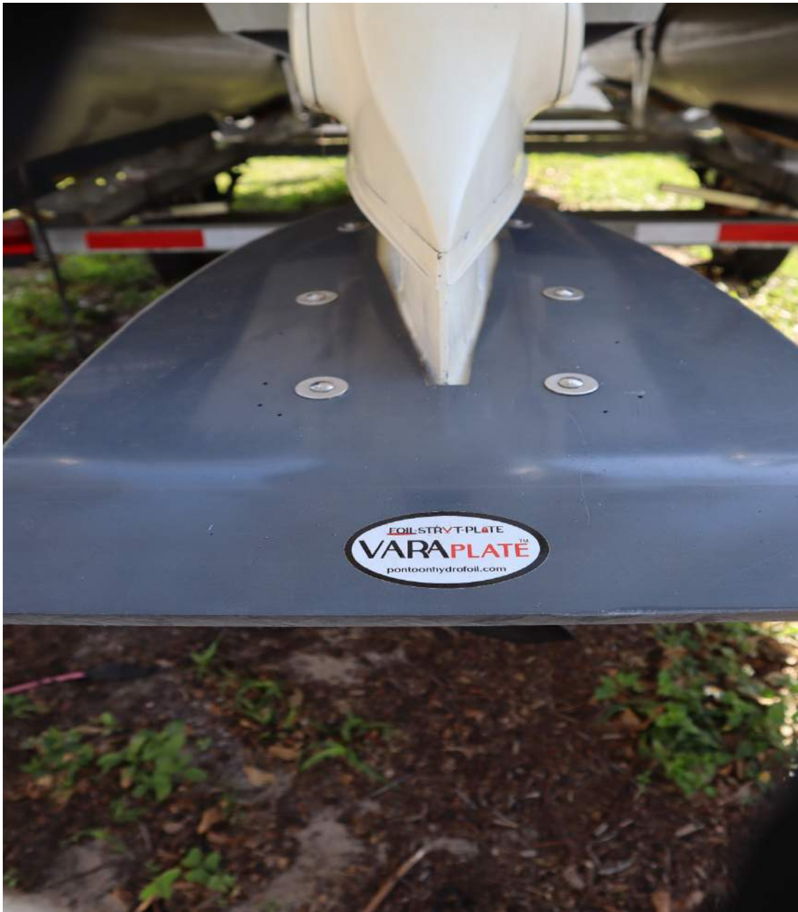
Top View: Note proper bolt alignment and pattern.
